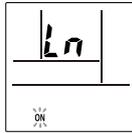
2. Press down **(BACK ON/OFF)** on the remote controller for more than 5 seconds.
