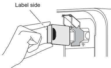
5. Close the WLAN adapter cover and the intake grille.
