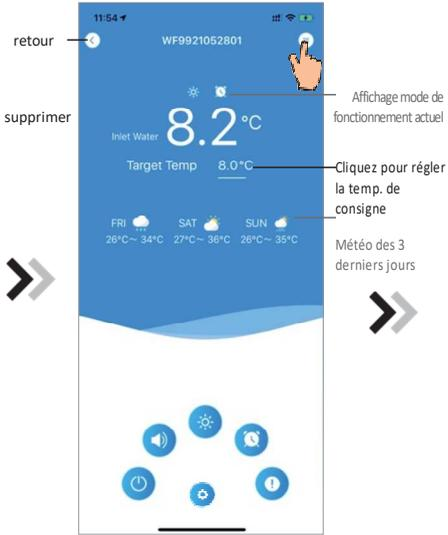
Fig.20 Interface principale appareil
